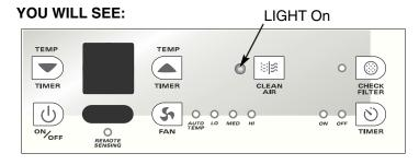
**Note:** When this feature is "ON", the electronic air purifier is energized to remove pollen and impurities from the air. To cancel this feature, press the Clean Air button (the LIGHT will turn off).
